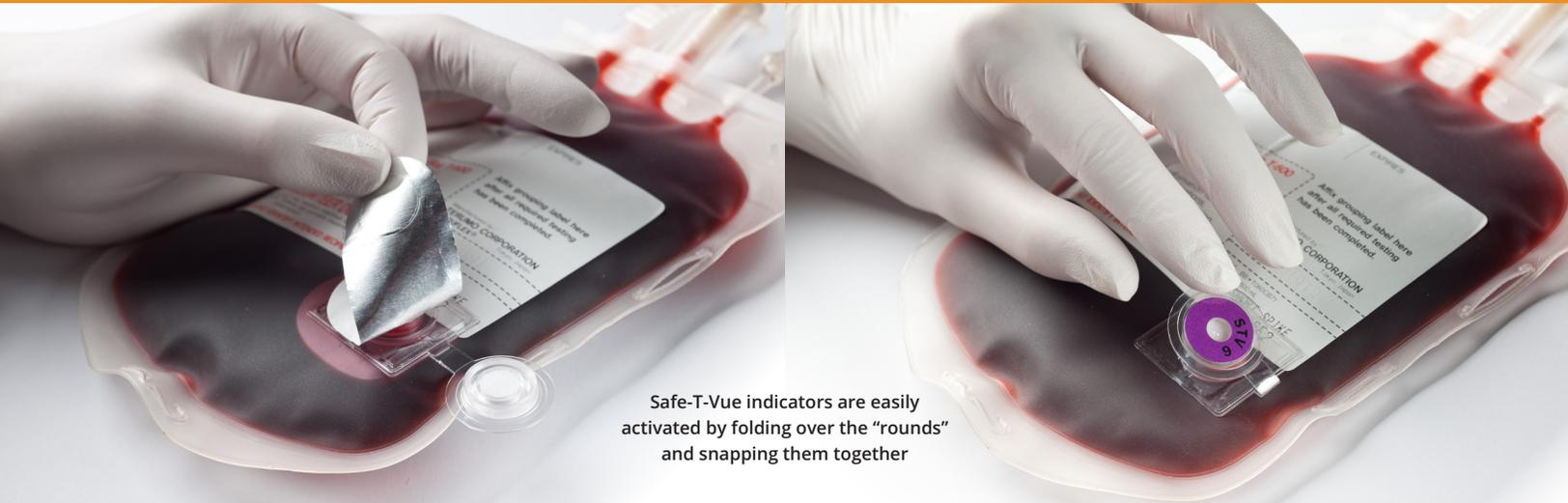
Safe-T-Vue indicators are easily activated by folding over the “rounds” and snapping them together
