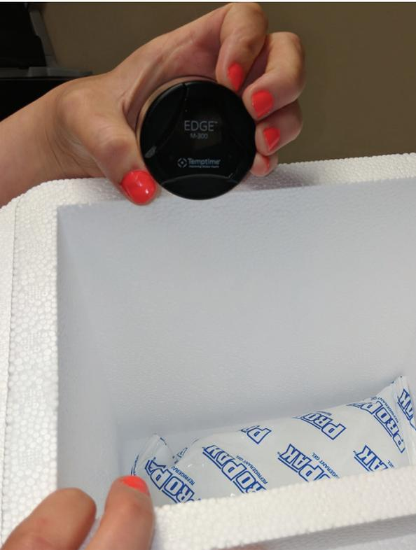
M-300 wireless sensors measured temperatures inside the medication packaging at regular intervals.
