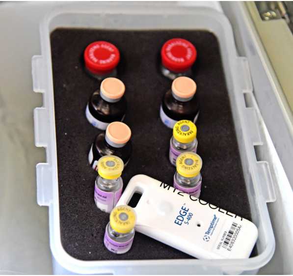
S-400 wireless sensor monitors medication in coolers onboard rescue vehicles.
