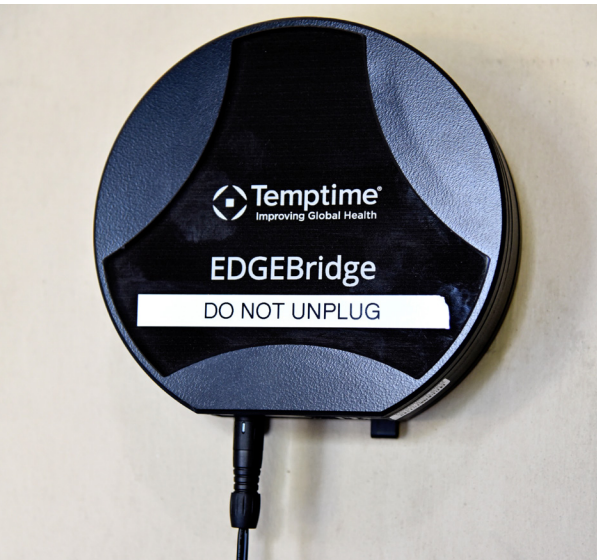
The wireless gateway is mounted on the station wall, and captures temperature data from the sensors as vehicles return to the stations
